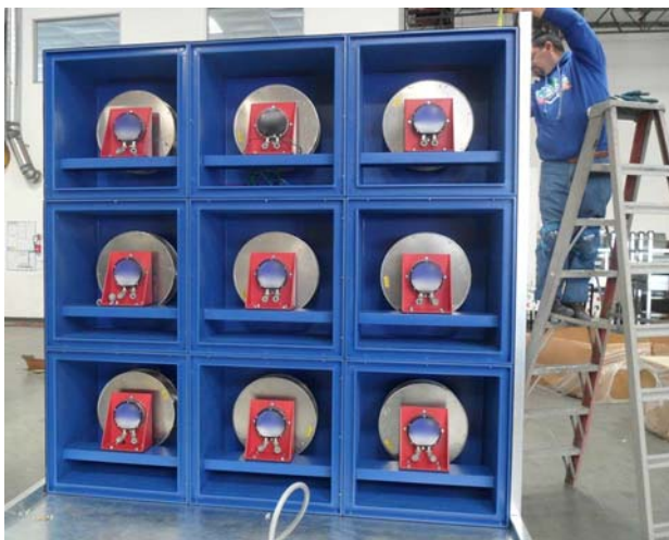
A 3x3 Multi Fan Unit designed to cool at 12,600 CFM
